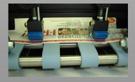
Straight Shooter introduced this revolutionary method of separation in 2004. Other feeders use a high friction "nip" point to separate documents. Straight Shooter eliminates the "nip" point for smoother feeding without the jams!
